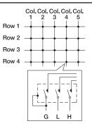
Each crosspoint in the matrix consists of a 3-pole Form A (normally open) relay. The shield of each relay is connected to the column GUARD line.
